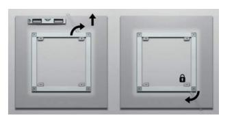
The frame hangs from the upper two Security Clips and the two lower Clips, once rotated using the Security Key, lock the frame into place.
